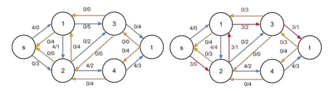
Left: An example of a residual network, blue edges are the original edges in the network, and orange ones are the reverse edges.
