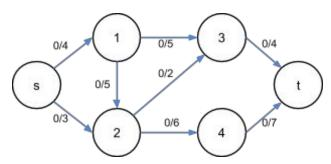
**Flow network** G = (V, E), V denotes the set of vertices and E denotes the set of edges, is a directed graph with each edge  $(u, v) \in E$  has a **capacity** c(u, v). There are two vertices that are distinguished from others, the **source** s and **sink** t, and every vertex  $v \in V$  exist a path in the flow network that goes  $s \to v \to t$ .
